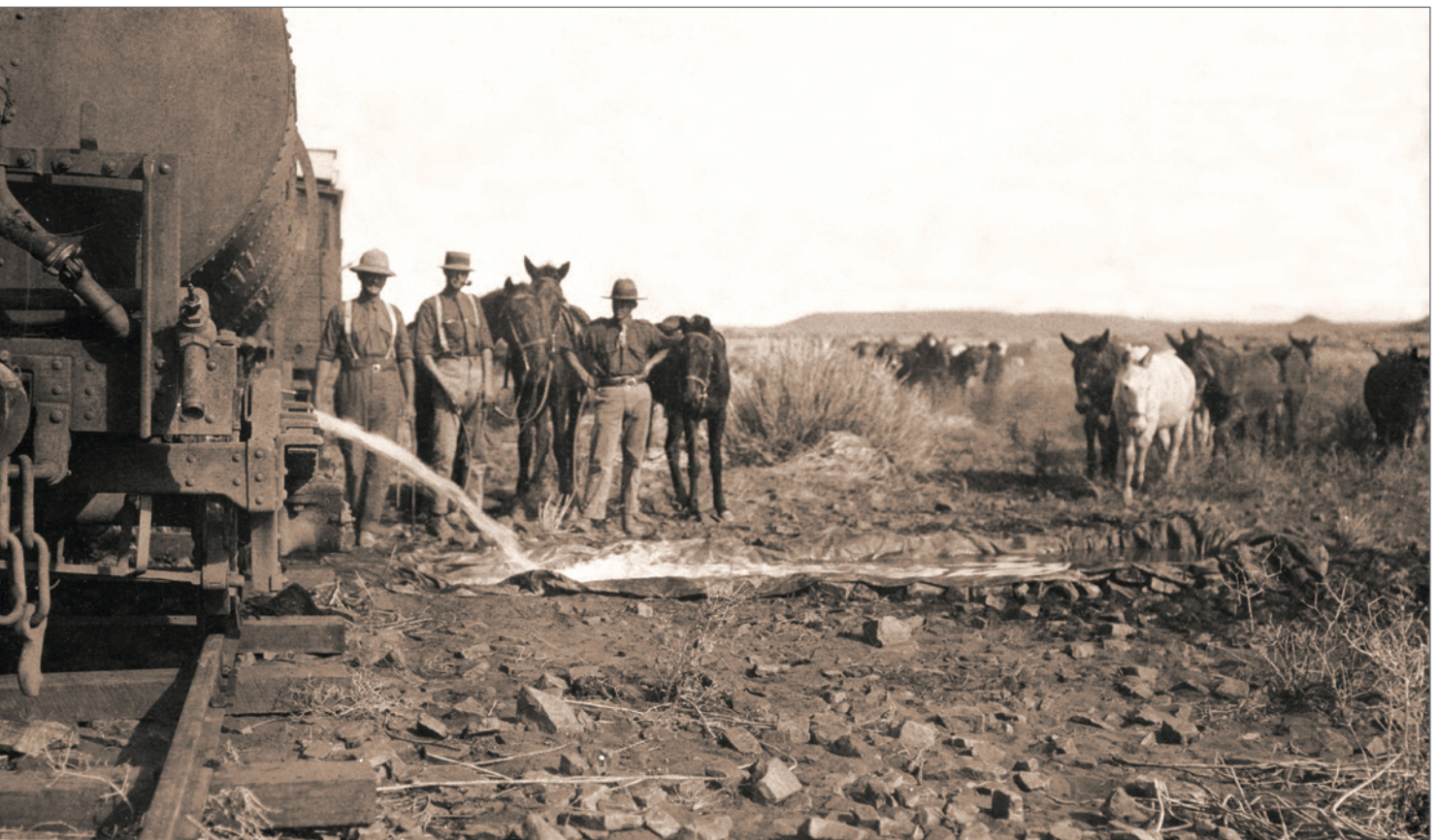
Figure 5: Water being discharged from a rail tanker into a temporary canvas-lined hollow for watering the mules (Transnet Heritage Library photograph GSWA017)
